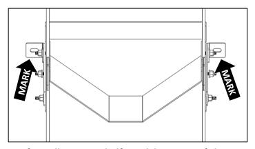
If installing onto shelf, mark locations of slots onto shelf side.
