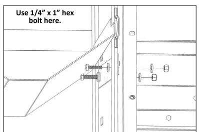
• For each tank tier, attach straps to loops on both sides of front of rack.
