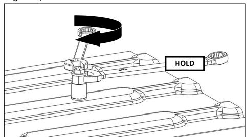
• Using the 9/16" box wrench, hold plus nut tool stationary to remove the 1/4" hex bolt.
