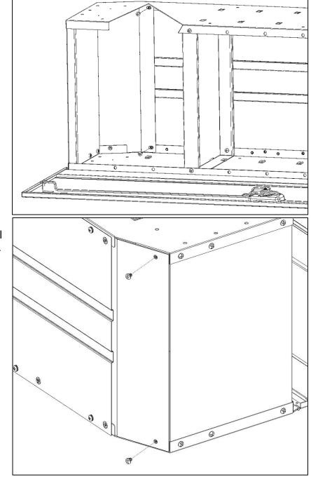
Install two 1/4" x 3/8" one-way screws through the rear cover panel into the top rear shelf panel flanges.
