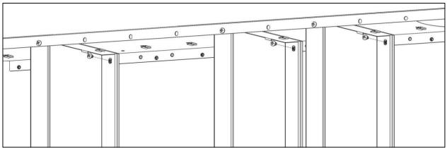
Making sure the shelves are square to the side panels, install the rear panel using fourteen 1/4" x 3/8" Phillips SEMS screws.
