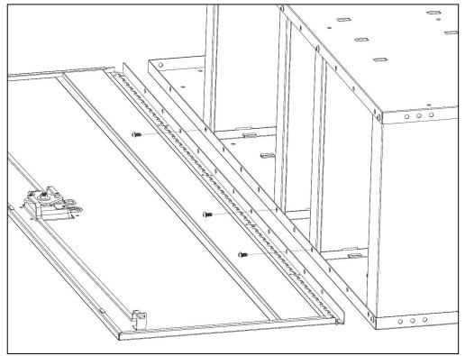
• Using eight 1/4" x 1/2" Phillips machine screws and eight 1/4" flanged lock nuts, install door to side panel.
