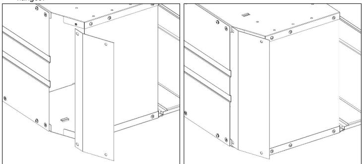
Install rear panel to the inside of the shelf-panel rear flanges using two 1/4" x 1/2" Phillips machine screws.
