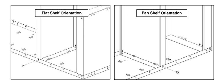
• Install one 1/4" x 1/2" machine screw through the rear of the shelf into the pressed-in nut on the rear of the shelf side.
