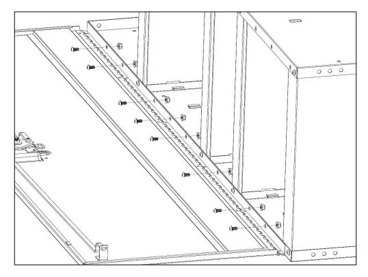
Install the top panel assembly using six 1/4" x 3/8" one-way screw.
