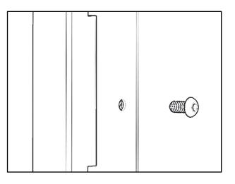
• On the attachment side, bolt together using a 1/4" flat washer and a 1/4" lock nut.
