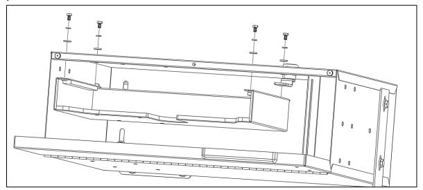
Using two #10 x 5/16" hex head bolts, two #10 lock washers, and two #10 washers, bolt the new file hanger to the laptop holder.
