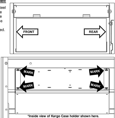
Using four 1/4 x 1/2" pan head screws, and four 1/4" flanged lock nuts, attach Kargo Case holder to shelf. Be sure to have screws facing down.
