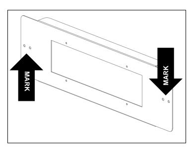
• Mark onto installation surface location of the two holes in the mount that best fit your vehicle.
