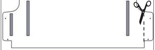
When installing 40475TL or 40476TL in Transit 148" wheelbase you must trim the rear floor section as shown for access to the spare tire mechanism.
