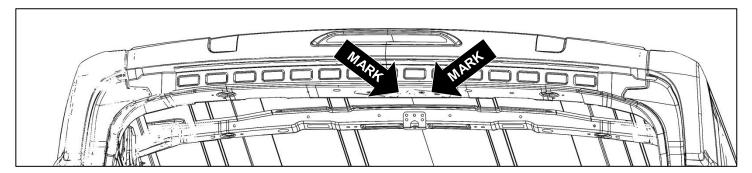
Hold second mounting bracket against the center of forward roof support beam. Be sure the
