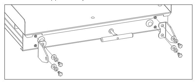
• Using two 3/8" x 1-1/2" button head screws, two 3/8" lock washers, and two 3/8" flat washers, install the pull handle assembly to the handle brackets. DO NOT overtighten.
