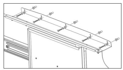
Reinstall D-rings through the slots in floor bracket.
