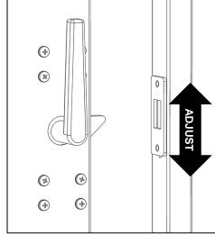
Using two #10 X 3/8" pan head screws, LOOSELY attach the driver side striker plate to the driver-side door jam.
