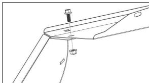
Using a 1/4" x 5/8" flanged bolt and 1/4" flanged lock nut, bolt corner panel to side wing.
