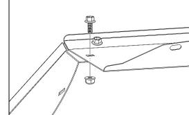
Using one 5/16" x 5/8" flanged bolt and one 5/16" flanged locknut, bolt corner panel to side wing.
