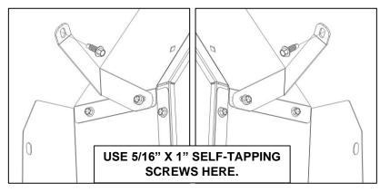
In the remaining locations along the wings, as shown, secure wings to the "B" pillars using 5/16" x 1" self-tapping screws.
