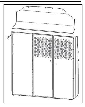
• Using six 1/4" x 5/8" flanged hex head screws and six flanged lock nuts, bolt the top wing to the top of the partition.
