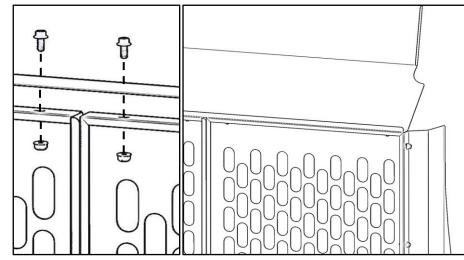
• Using five M8 x 25mm hex head screws, five 5/16" lock washers and five 5/16" flat washers, bolt the top wing into the threaded embosses across the roof support in orientation shown.
