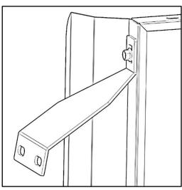
• Using a M8 x 25mm hex head screw, a 5/16" lock washer and a 5/16" flat washer, bolt the other side of the bracket into the threaded embosses in the side of the van in orientation shown.
