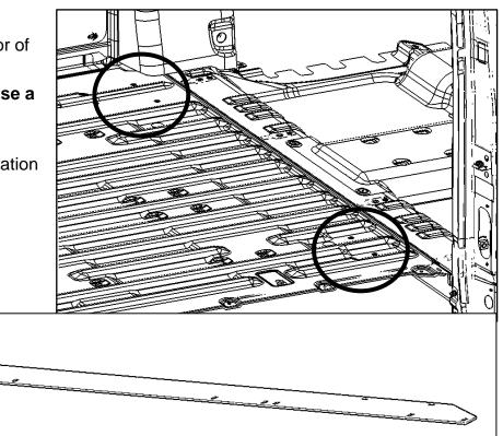
• Using a M8 x 50mm hex head screw, a 5/16" lock washer and a 5/16" flat washer, bolt to floor in orientation shown.
