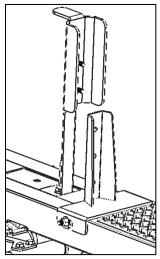
Remove the 3/8" x 1" hex head bolt, two 3/8" washers, and the 3/8" lock nut and remove the ladder hook.
