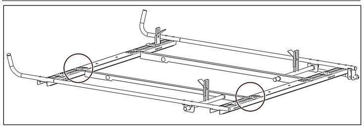
• Attach the long L-bracket to both bows in the orientation shown using 3/8" x 1" carriage bolts, 3/8" flat washers and 3/8" lock nuts.
