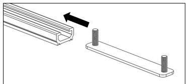
• Feet may be mounted inward or outward. Feet will face inwards on standard low roof installations and will face outwards on all high roof installations.
