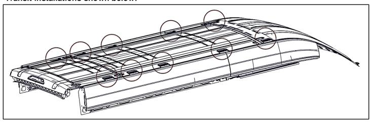
• Use the dimensions (X & Y) measured from the roof mount locations and coordinate onto the rack crossbars. Some slight adjustment will be available once rack is placed onto roof.
