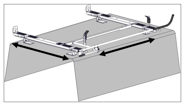
• Mark four locations at each foot mount location onto the top of the shell.
