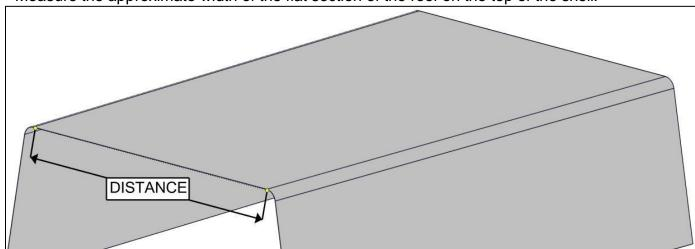
Determine best mount locations on top of the shell and measure distance between the desired mounting locations.
