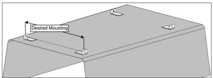
At the width desired, find the corresponding slots on the ladder rack cross bow and attach mounting feet as shown.
