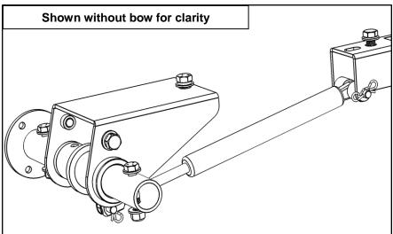
Note: In some situations, you may be easier to wait until handle assembly is installed to attach both ends of the damper. This is so you can use the handle to help shorten the distance between the two ends the damper.
