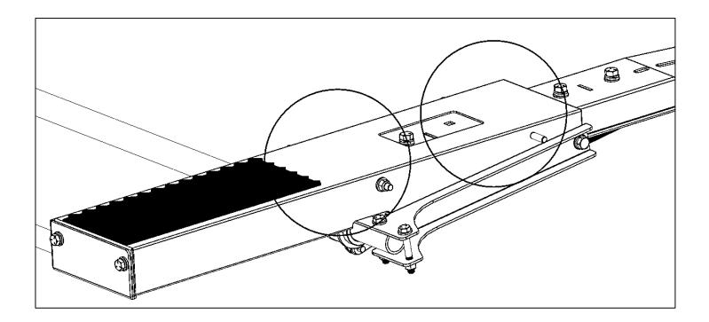
• Typically, the ladder hook on the front bow is installed on the threaded stud closest to the end of the bow.
