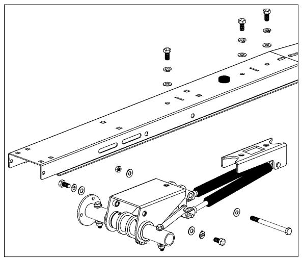
• While installing the 3/8" x 4-1/2" hex head bolt, **be sure to NOT lose the pre-assembled nylon washers.** These nylon washers go to the inside of the bow.
