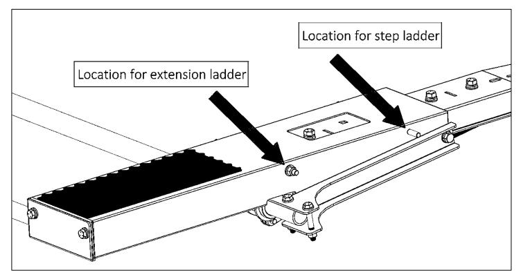
When using an extension ladder, place the ladder hook at the threaded location closest to the end of the pan.
