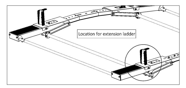
• When using a step ladder, place the ladder hook at the threaded location closest to the center of the bow.
