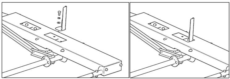
• Bolt Ladder Hook (H) to the lower position where the pem studs are installed. Use a 5/16" flat washer (6) and a 5/16" nyloc nut (9).
