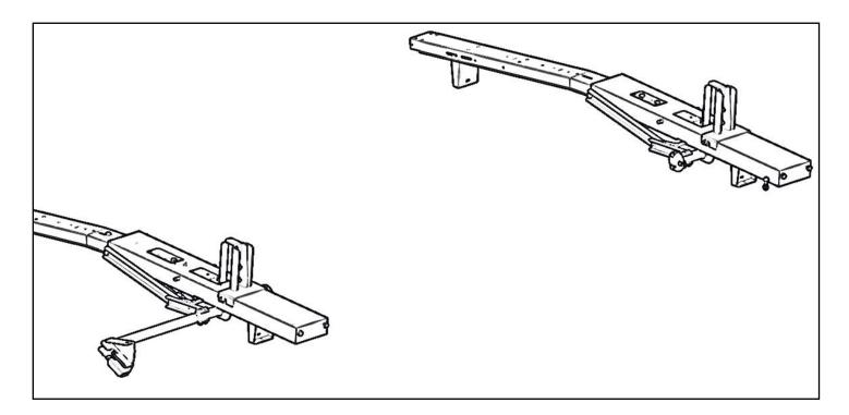
Bolt Torque Tube (C) to Rear Bow Assy (B) using three 1/4" x 7/8" hex head bolts (5) six 1/4" flat washers (3) and three 1/4" nyloc nuts (4).
