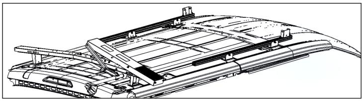
Place a foam block from the packaging to hold the bow in the up position in order to access the mounting slots.
