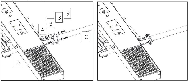
• Repeat process to bolt to the front bow assembly (A).
