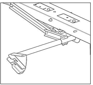
If installing on a High Roof Extended Transit, the Handle Extension (L) will be used.
