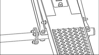
• Using three more 1/4" x 7/8" hex head screws, 1/4" washers, and 1/4" lock nuts, attach the opposite end of the torsion tube extension to the torsion tube as shown below.
