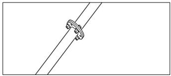
• Using three more 1/4" x 7/8" hex head screws, 1/4" washers, and 1/4" lock nuts, attach the opposite end of the torsion tube to the rear bow as shown below.
