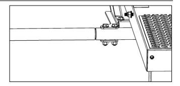
Attach handle into operator arm by pushing handle in and then pulling out.
