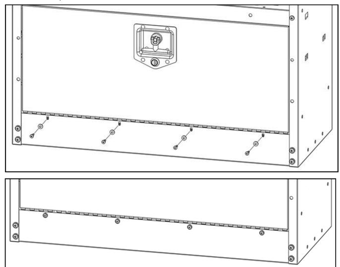
Square and align door kit before tightening hardware.
