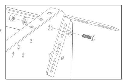
Using one 1/4" x 7/8" bolt, two 1/4" flat washers, and one 1/4" lock nut, bolt the L-mounting bracket to the rear pillar unit. There are existing holes in the rear pillar of the van that can be utilized. The picture shows a 46" high shelf installation. If installing a 43" high shelf, use the lower slot on the L-mounting bracket.
