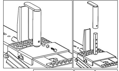
• Remove the 3/8"-16 x 1" hex head bolt, two 3/8" washers, and the 3/8"-16 lock nut and remove the ladder hook.
