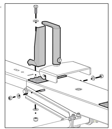
Where the ladder stop is removed, replace hardware and tighten.
