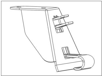
• LOOSELY bolt the gutter clamp to the gutter foot using a 5/16" x 1-1/4" carriage bolt, 5/16" flat washer, and 5/16" lock nut. **DO NOT TIGHTEN**.
