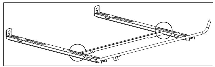
Insert the plastic bushings into the clamp and lock L bracket and angle bracket installed in Step 5, with flange towards each other and to the inside as shown.
