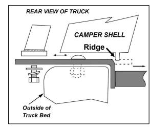
locations on the top of each mount plate. The bolts should be located as far apart as possible, with clear access to the bolts, washers, and nuts underneath the truck's bedrail.
