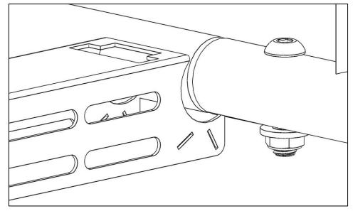
• Insert a side channel clamp into cutout in each crossbar with interior diameter facing upward.
