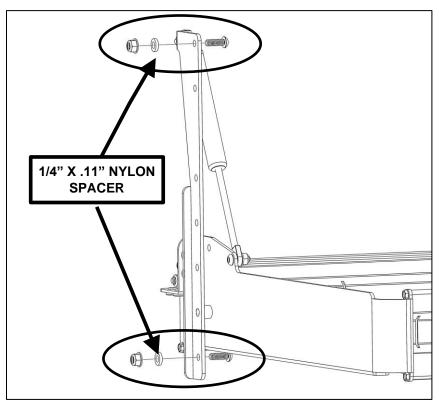
The lower button head screw head is accessible through the 3/4" hole in the side of the shelf.
