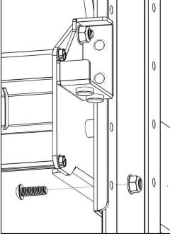
Again, for ease of tightening, the lower button head screw head is accessible through the 3/4" hole in the side of the shelf.
