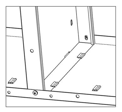
NOTE: The ProMaster requires the lowest shelf be raised by one set of lances to clear the wheelwell. Image on the left reflects most applications. The image on the right shows the bottom shelf for a Ram ProMaster.
