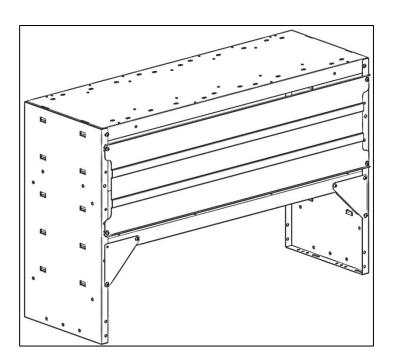
When installing the rear panels to the shelf assemblies, be sure the single lip flange is facing away from the shelf. If the rear panel is installed incorrectly, it may cause a rattle noise.
