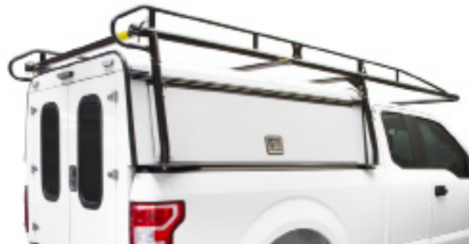
PRO II Heavy-Duty Steel Cargo Rack for Full Size Trucks (2" Dia.) 1,700 lb Capacity – Black
