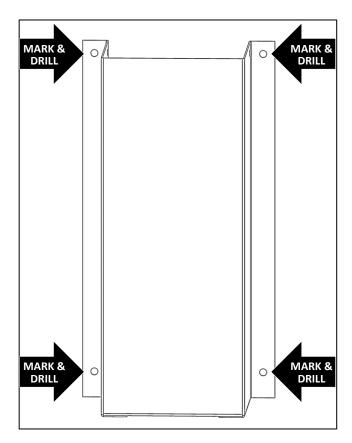
NOTE: If installing reflector kit holder to a partition, be sure screw head is on cab side.
