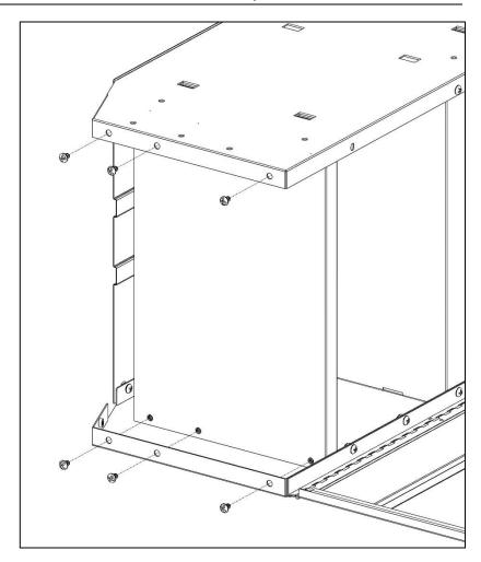
• Slide the rear cover panel inside the shelf-panel rear flanges and outside the top rear shelf-panel flanges.
