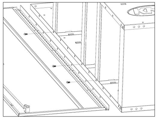
• Using eight 1/4" x 1/2" Phillips machine screws and eight 1/4" flanged lock nuts, install door to side panel.
