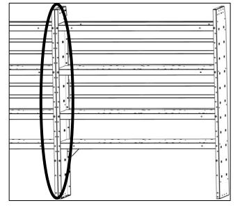
Using one 1/4" Phillips pan head screw, two 1/4" flanged hex head screws and three 1/4" flanged lock nuts, bolt center conduit carrier mount to the center rear shelf end panel. Repeat for each additional 40235 installed.
