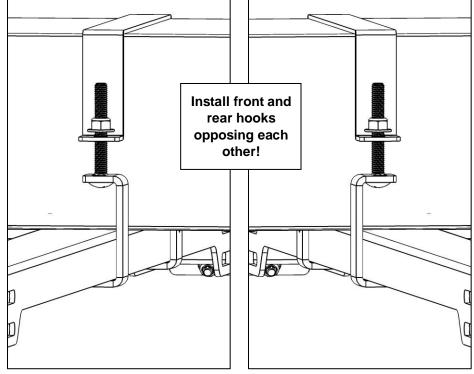
• Tighten the nuts on the bolts connecting the mounting hooks to the mounting brackets.
