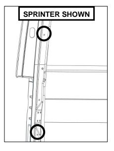
Grab handle can also be mounted to shelf end panels, van partitions and GM vans by drilling mounting holes. Some sample installations shown below.
