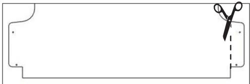
When installing 40475TL or 40476TL in Transit 148" wheelbase you must trim the rear floor section as shown for access to the spare tire mechanism.
