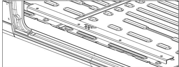
• While applying firm pressure against threshold, mark the four holes onto the floor or floor mat.
