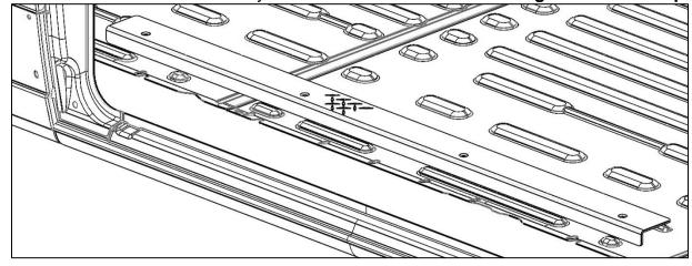
• While applying firm pressure against threshold, mark the four holes onto the floor or floor mat.
