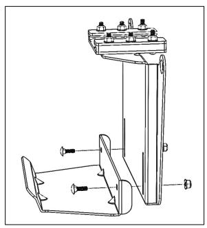
With hook pointed towards rear, slide slots in sliding hook assembly over rail flanges at forward end of rail assembly.
