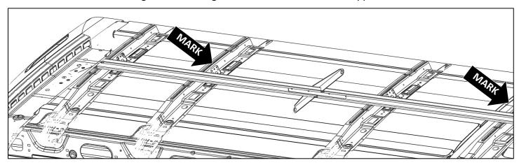
• Make a mark on rail 11" from the rear of van interior ceiling. This mark will be needed during assembly.
