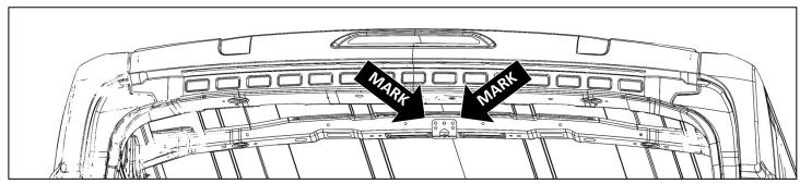
• Hold second mounting bracket against the center of forward roof support beam. Be sure the mounting bracket is level to the roof support beam. Mark mounting hole locations on the roof support beam.
