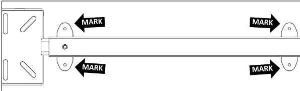
Move the vise mount assembly out of the way to show the marked locations.
