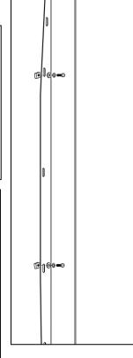
• If factory D-rings were factory installed and previously removed from "B" pillar, re-install D-rings through slots both driver side and passenger side of floor bracket.
