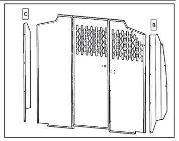
Bolt together using a 1/4" x 5/8" flanged hex head and a 1/4" flanged nyloc nut.
