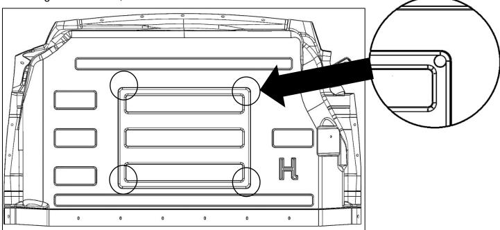
• Using a jigsaw, cut a straight line from each hole previously cut, so that you have a square hole that fits the window accessory.
