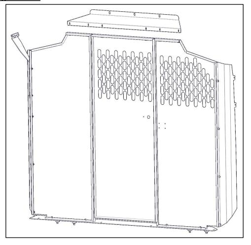
Bolt into the top of the partition using 1/4" x 5/8" flanged HH (5) and a flanged nyloc nut (7).
