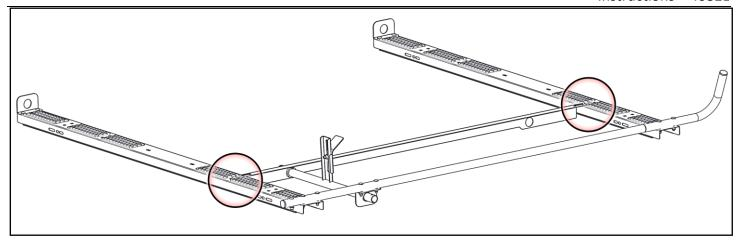
• Attach the long angle bracket to both bows in the orientation shown using 3/8" x 1" carriage bolts, 3/8" flat washers and 3/8" lock nuts.
