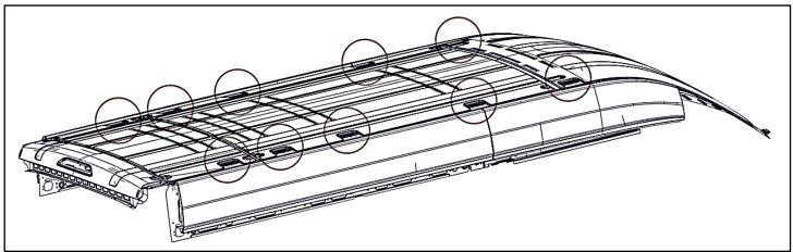
• Use the dimensions (X & Y) measured from the roof mount locations and coordinate onto the rack crossbars. Some slight adjustment will be available once rack is placed onto roof.
